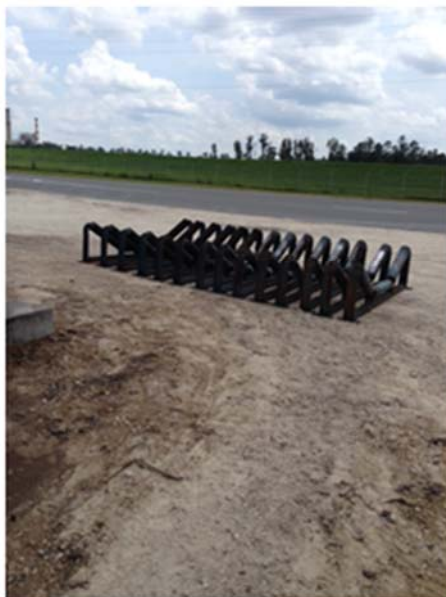
Rollers removed from #4 belt
