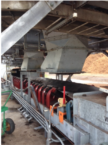
#9 conveyor side plates removed for replacement, both sides
